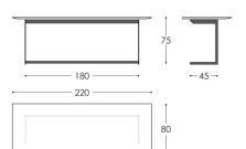
Working table. Rectangular top, 30 mm of thickness. Metal structure lacquered.
